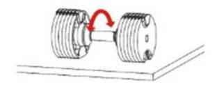
Place FLEXBELL on flat surface. Try turning the handle with normal force. The handle must remain in locked position. Check that the bar ends are within 5mm of the selected plate.
