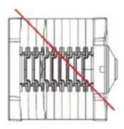
Make sure that the Male/Female connectors are aligned. Do not use if connectors are damaged.
